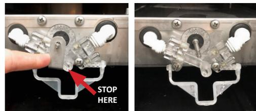
NOTE: Hands covered with cut resistant gloves can be used in place of the tool to turn shaft. Turn shaft until one of the edges/tines on the shaft is aligned at top of shaft.
