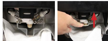
NOTE: Do not force the latch over the pump, if the latch does not snap into place adjust the motor shaft until the pump properly seats on the sanitation fitting and latches easily. See section MOTOR SHAFT ALIGNMENT for how to adjust motor shaft.
