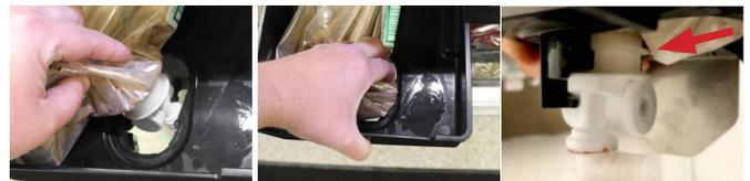
10. Slide the loaded product bin into correct slot in the lower refrigeration cabinet and latch into place.
